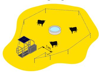
Introduce the Autonomous Weighing (WOW) system leaving a 1m opening to the non-Tru-Test Large antenna side. This allows cattle free choice to enter/exit via the WOW system or the 1m opening.
