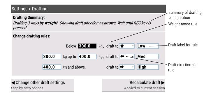
When drafting is enabled and **Show draft direction on Weigh screen** has been enabled during Step 1 of the drafting setup wizard, the **Weigh** screen will display the draft direction on a section of the screen. This also includes the count for each sort direction or pen, each with a label:
