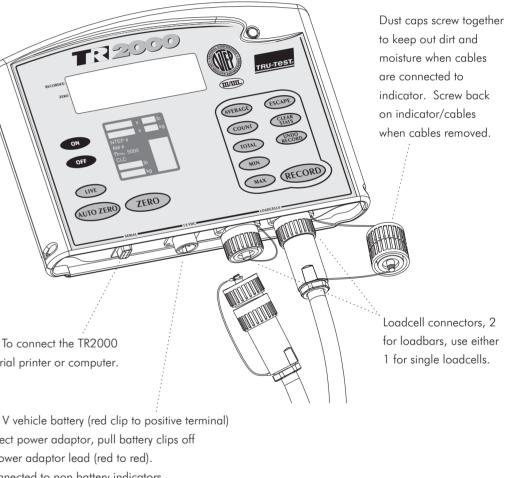
Serial port. To connect the TR2000 to a serial printer or computer.
