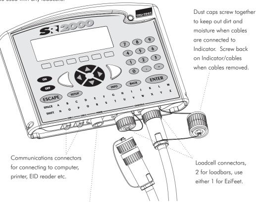
Power connector for connecting 12 V vehicle battery (red clip to positive terminal) or Tru-Test power adaptor.
